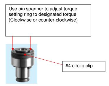
How to adjust the torque on adjustable tap collet:
